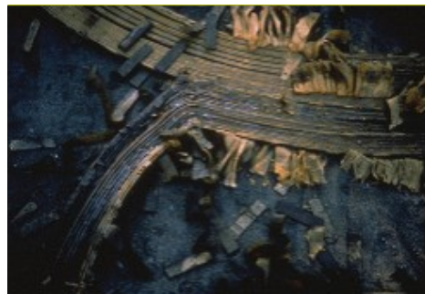
Figure 2-3. GIC Damage to Transformer During 1989 Geomagnetic Storm
