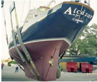
Full-bodied hull with full-length keel and propeller set in an aperture – water speed into prop reduced by as much as 40% in this case.
