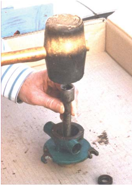
Using a 'drift' to punch out the bearings and seals
