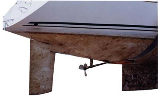
Well-exposed propeller with a long-fin keel and a moderate hull – water speed into hull reduced by about 20 to 30%
