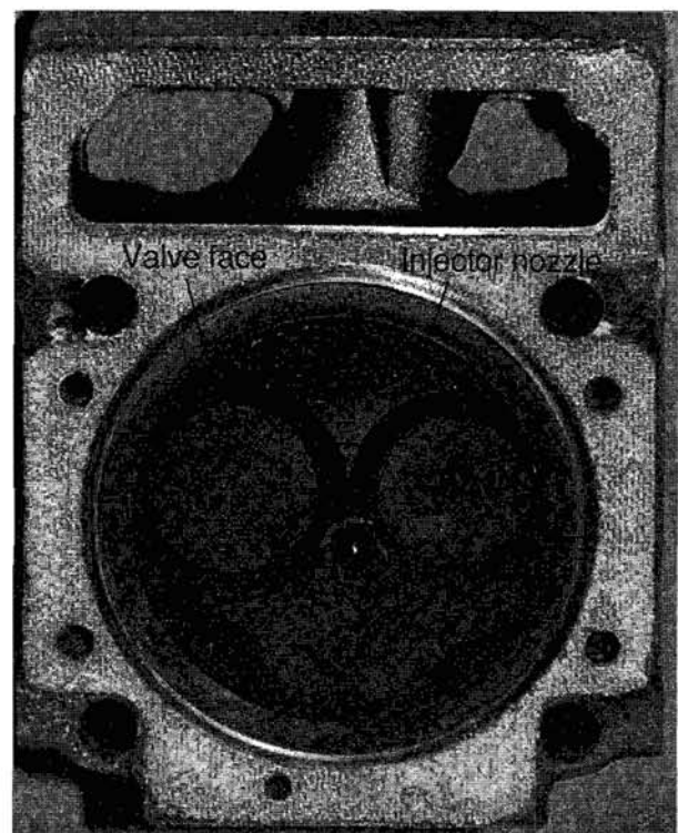
Figure 11-12. A cylinder head removed (Volvo MD17C). Care must be taken not to rest the head on the injector nozzle. (Note that this is a direct combustion chamber engine; therefore there is no precombustion chamber in the cylinder head.)
