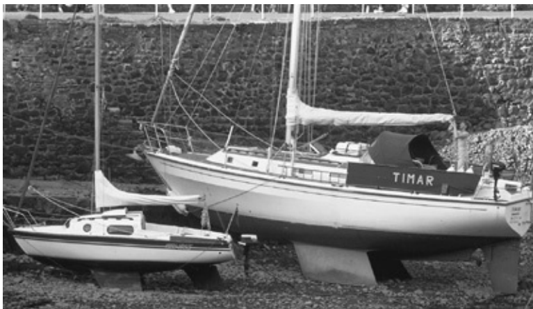
An interesting keel variant: twin bilge keels designed for drying out in tidal waters.
