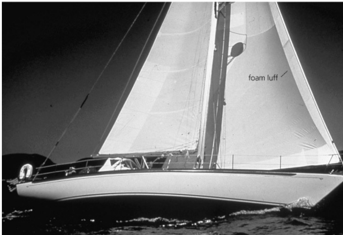
The padded foam luff on this roller-reefing headsail will help to flatten the sail when it is partially rolled up. (Courtesy Harken)
