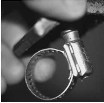
400-series stainless steel is highly magnetic.
