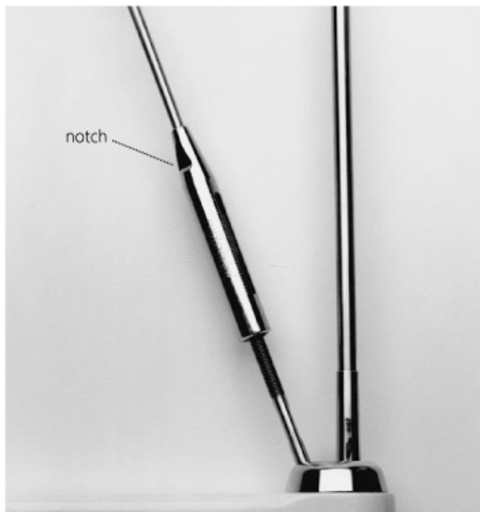
Discontinuous rod rigging, utilizing fatigue-indicating fittings (the long, tapered sleeve with a notch in it; the sleeve will break before the fitting fails, providing an early warning of impending trouble). (Courtesy Navtec)
