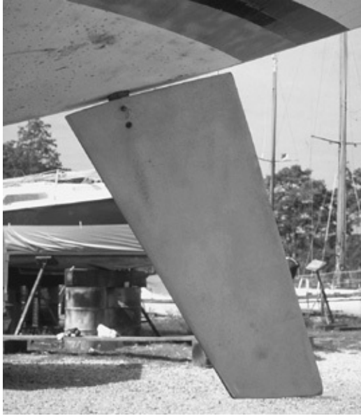
Spade rudder. Excellent performance, but limited strength in a grounding.
