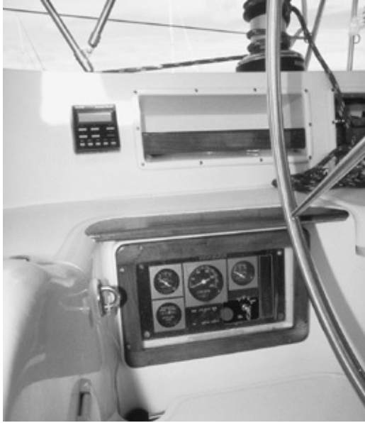
Nada's engine panel, in the side of the cockpit well. I should have had it moved at least to the coaming, and preferably to inside the boat.
