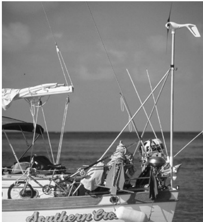
An incredibly elaborate custom-made pushpit that includes mounts for a wind generator, solar panels, a radar, various antennas, an outboard motor and crane, a Lifesling, another rescue throw device, a stern anchor, fishing poles, and probably several other things I have missed!
