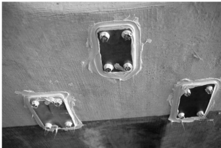
Substantial backing plates spread hardware stresses and minimize the chance of leaks developing. My preference is to not bed the backing blocks. This way, if a leak develops at the deck level, it is possible for the water to make it into the boat and sound the alarm, rather than being trapped in the core.
