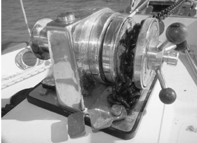
Chain rodes build up steep-sided cones, which then jam the naval pipe (left) and the windlass (right).
