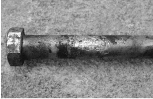
Stainless steel bolt with active galvanic corrosion cell (the shiny metal).
