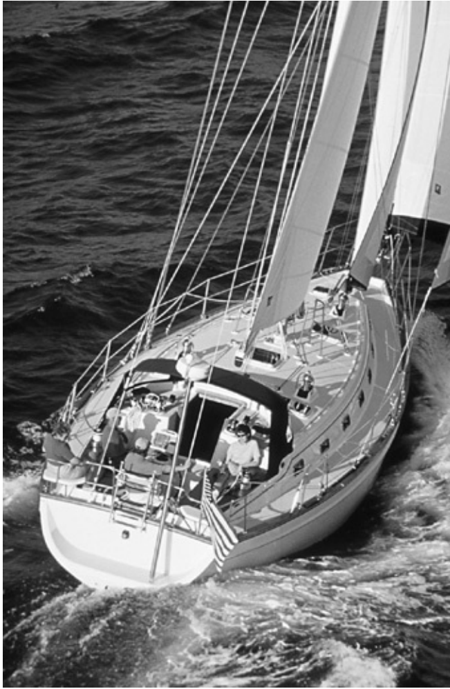
Island Packet 420, a moderately heavy-displacement cruising boat, close reaching at 8 knots (speed–length ratio of about 1.3). The boat is sailing pretty much on its quarter-beam buttock line; the stern wave is starting to crest right at the transom. (Courtesy Island Packet)
