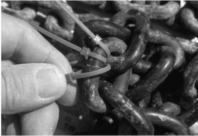
Using tie-wraps to mark a chain.
