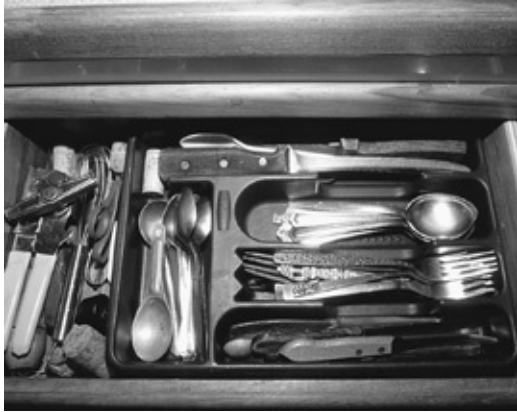
Cutlery stowage on Nada. This is the drawer with two drawer pulls—it is difficult to open single-handedly, which is annoying in rough conditions.
