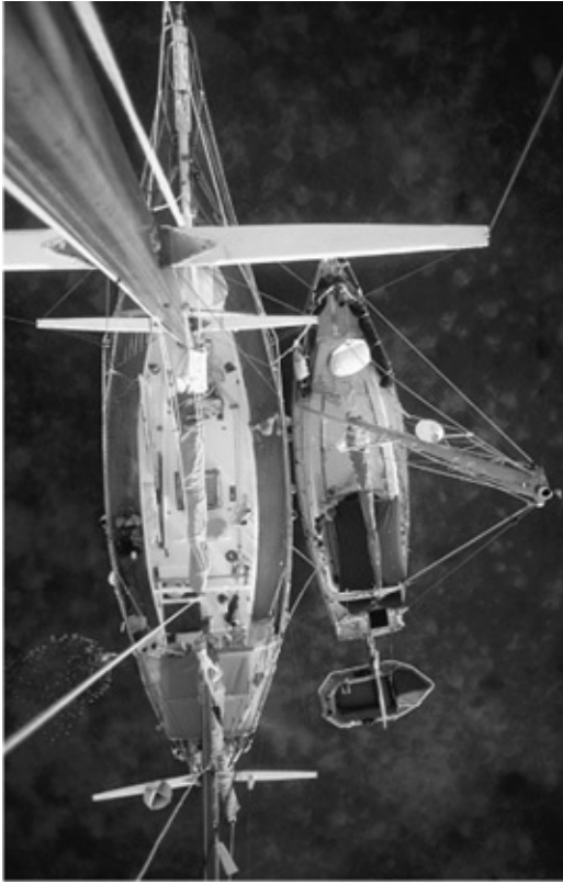
Rafting up. Large fenders and plenty of spring lines are needed, together with staggered masts and rigging.
