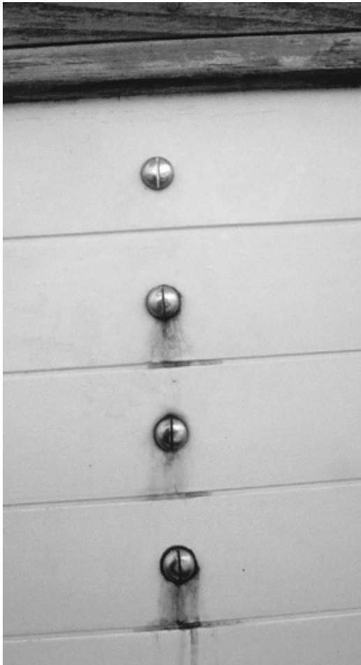
Rust stains emanating from a series of chain-plate bolts; these are almost certainly not just cosmetic stains.
