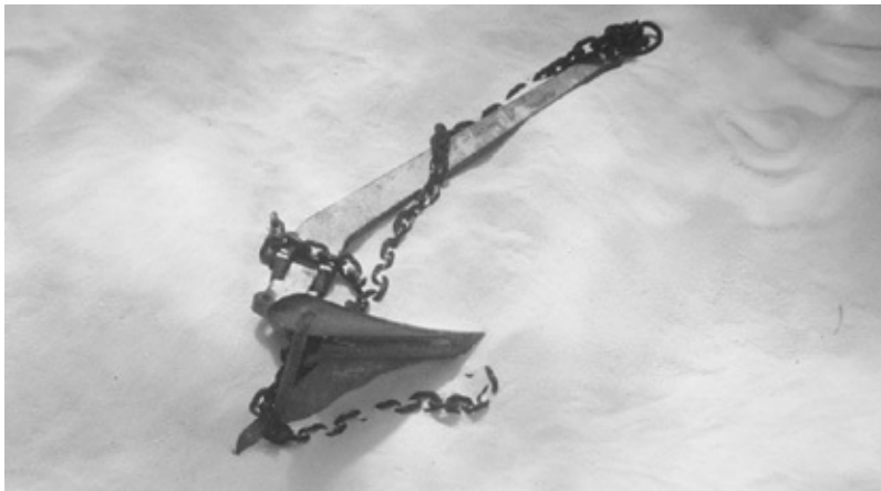
If the anchor rode is let out in a hurry, it may pile up on the anchor and foul it (especially a Danforth-type anchor).
