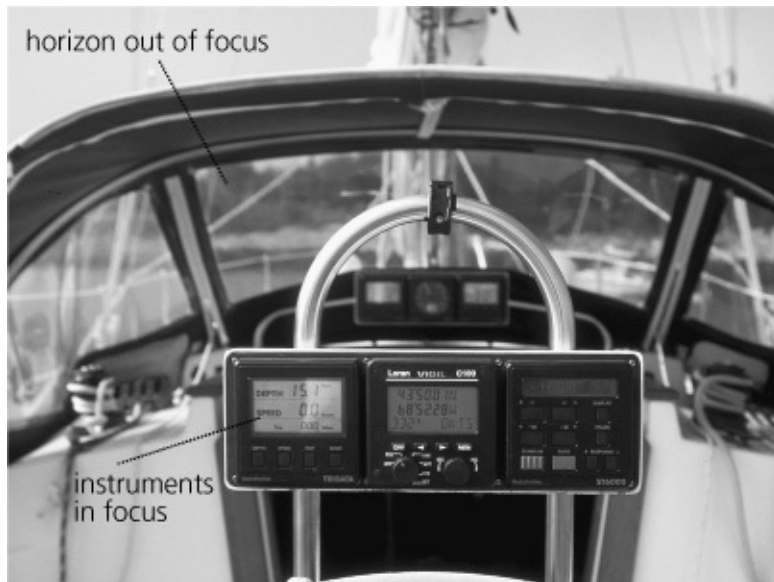
Pedestal-mounted instruments: note how it is necessary to refocus to read the instruments and look in the distance, whereas this is not necessary with instruments mounted over the companion-way (which, unlike the binnacle-mounted instruments, are also visible from other watchkeeping stations).
