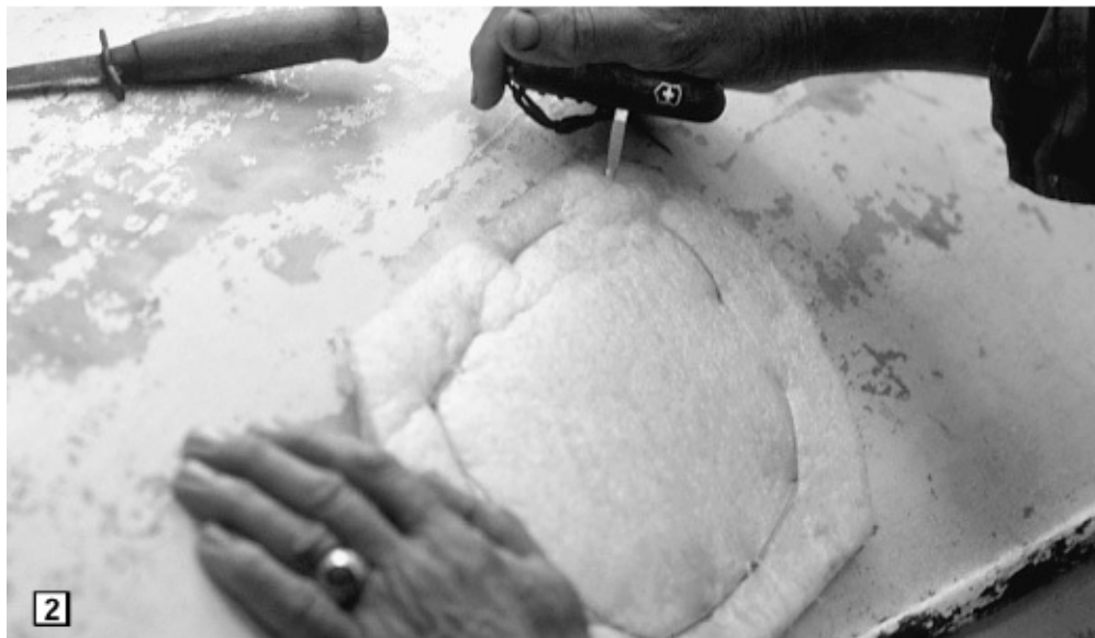
1. A submerged log punched a fist-size hole in the dinghy way up a jungle river in Guatemala, miles from anywhere 2. We temporarily patched it by stitching on the lining from a cockpit cushion. You can't do this with an inflatable!
