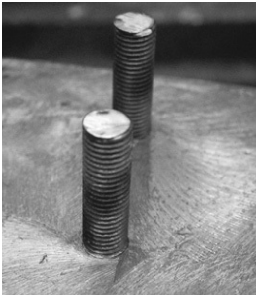
Stainless steel J-bolts cast into Nada's keel: I much prefer to see the bolts installed in a way that makes them removable.
