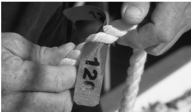
Installing rode markers in a nylon rode.
