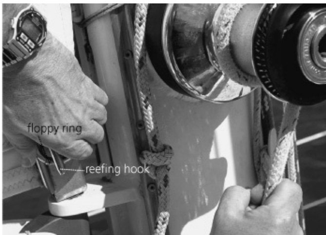
Reefing hook in action—the halyard is eased sufficiently to enable the floppy ring attached to the tack cringle to be pulled over the hook.
