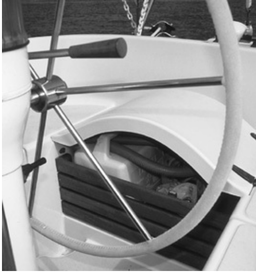
A neat solution to the stowage of gas cans, which otherwise tend to get tied down on deck.
