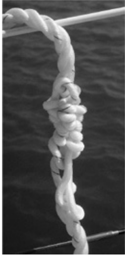
Top: Three-strand rope construction. (Courtesy New England Ropes). Above: Minor (left) and severe (right) hockling. The former can be worked back into the lay of the rope without damage; the latter is impossible to fully restore—some degree of permanent damage has occurred.
