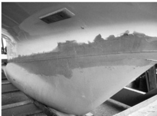
Nada's keel being installed. Note the swept-back leading edge, the rounded toe, the wide root area (which spreads the shock load of a grounding), and the sloping angle at which the keel joins the boat's keel stub (which also helps spread shock loads to the hull without unduly stressing the keel bolts): all are desirable features in a cruising boat.
