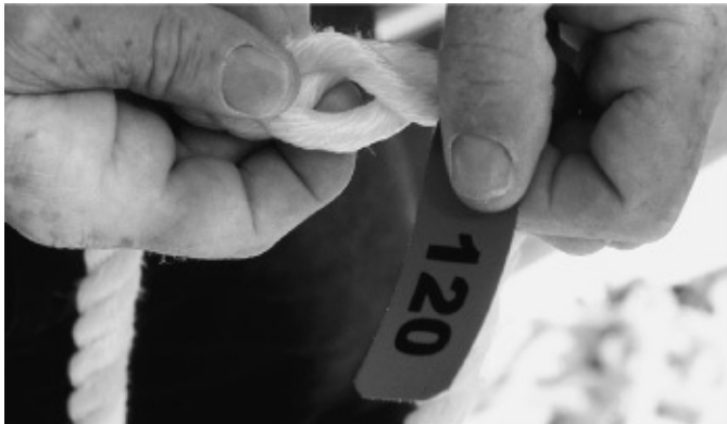
Using tie-wraps to mark a chain.
