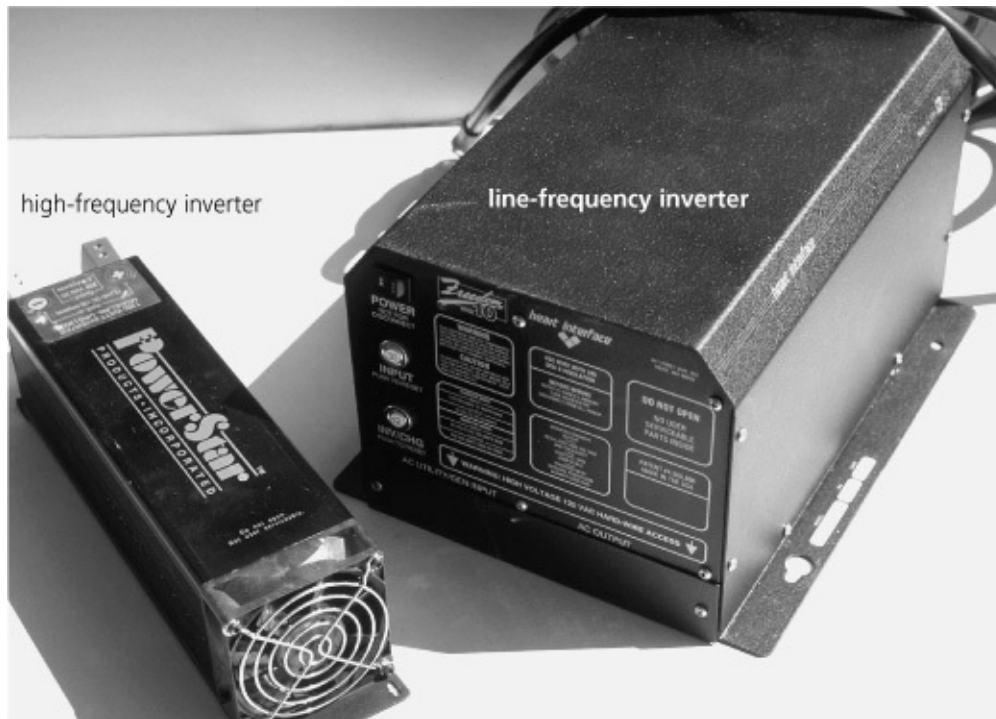
A 1,000-watt high-frequency inverter versus a line-frequency inverter. Note the difference in size (there's also a weight difference). However, the line-frequency inverter can be used as a battery charger, whereas the high-frequency inverter cannot (some can); there are other subtle differences that affect choices.
