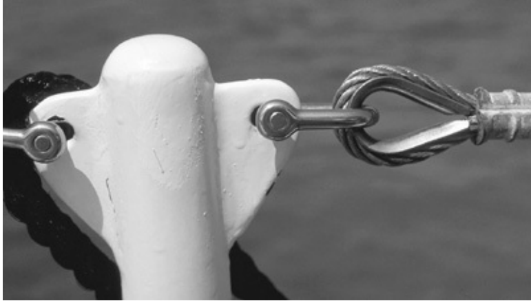
Solid plates welded to the stanchions for lifeline attachment—in this case, on a steel boat—but it can just as easily be done with stainless steel stanchions.
