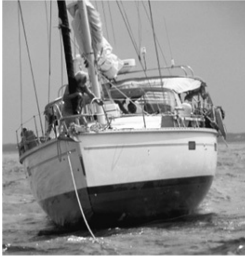
A wing-keeled boat stuck on a coral reef. It proved extremely difficult to get off, and was ultimately rescued at the expense of the wings on the keel.
