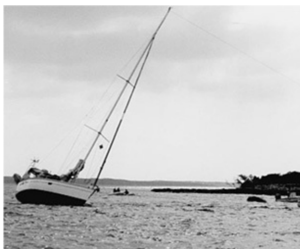
Above left: Pulling a boat down by the masthead. This effort was ineffective because the anchor was set way too close to the boat. Above right: Wing-keeled boat aground on a reef. It was pulled down by the masthead until the side decks were submerged. The wings bent up and the boat was jerked off with no other damage. Note the masthead bending on this fractional rig. We had some concerns that we would buckle the mast at the cap shrouds, but the situation was desperate enough to take the risk. (Courtesy Heidi Rabel)
