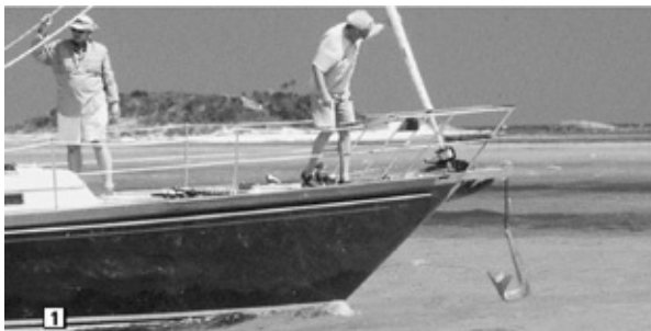
If the anchor rode is let out in a hurry, it may pile up on the anchor and foul it (especially a Danforth-type anchor).
