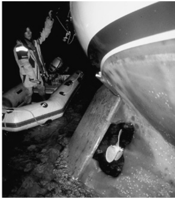
The keel and skeg arrangement on Nada is such that however distressing a grounding such as this may be (Terrie is looking a little stressed out!), little or no damage will be done to the boat.
