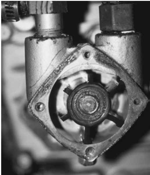
Damaged raw-water pump impeller. As is often the case, the engine was still running fine (most engines have excess cooling capacity in normal circumstances). This kind of damage is only found through regular inspections.
