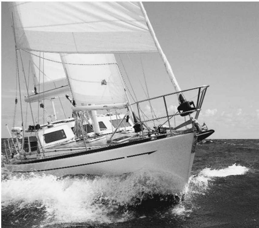
Cutter reefed down. The next step is to roll up the headsail altogether and reef down the main some more. (Patrick Parsons photo, courtesy Harken)
