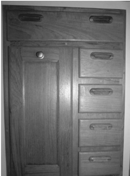
Single and double drawer pulls. The top drawer, with two drawer pulls, is difficult to open one-handed underway. A single pull in the center of the drawer does not look as elegant, but is more functional.
