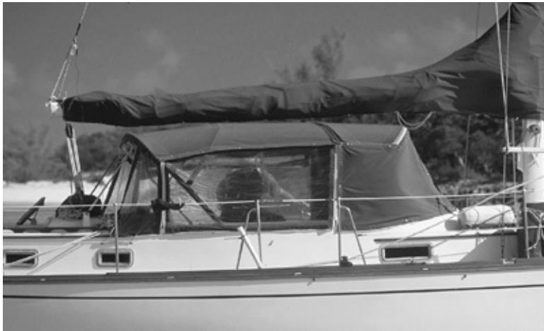
Note the covers on the front of this dodger, which reduce the greenhouse effect and extend the life of the clear plastic (which suffers from UV degradation over time). This is a 40-foot center-cockpit boat that manages to maintain attractive lines—quite an achievement.
