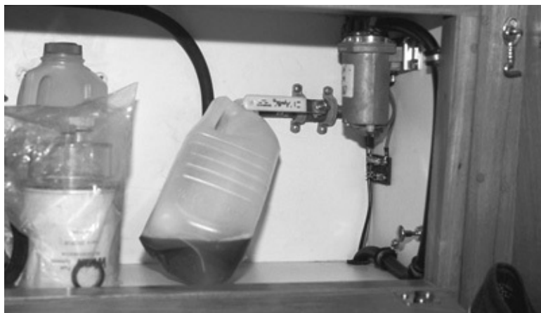
Nada 's fuel-sampling system. The pump is plumbed to a low spot in the tank.
