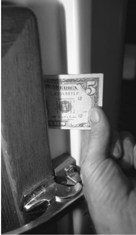
Testing the seal on an icebox door.
