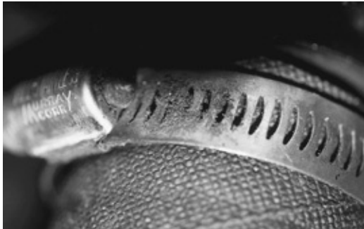
All-stainless-steel hose clamp freely corroding. The screw is made from 400-series stainless steel.
