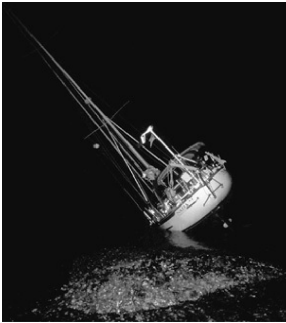
The keel and skeg arrangement on Nada is such that however distressing a grounding such as this may be (Terrie is looking a little stressed out!), little or no damage will be done to the boat.
