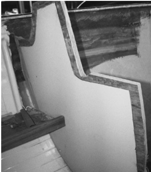
Bulkhead on Nada being prepared for bonding to the deck structure.
