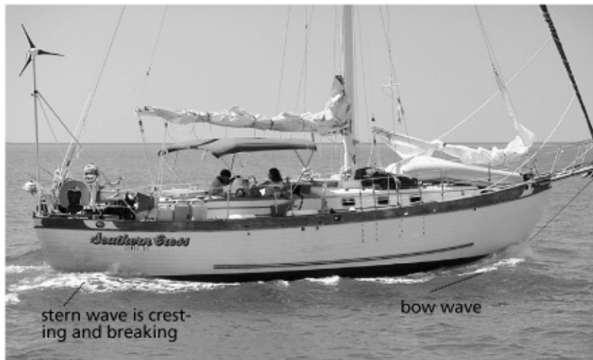
A 43-foot (13 m) double-ender doing 6½ knots (speed–length ratio of about 1.2). Despite having a similar LWL to the Catalina 42 and a longer LWL than the Saga 35, and traveling a knot or more slower, the lack of buoyancy in the stern and quarter-beam buttock lines that angle sharply upward are causing the boat to squat and make considerable waves. It will take a huge amount of power to get this boat up to 8 knots.
