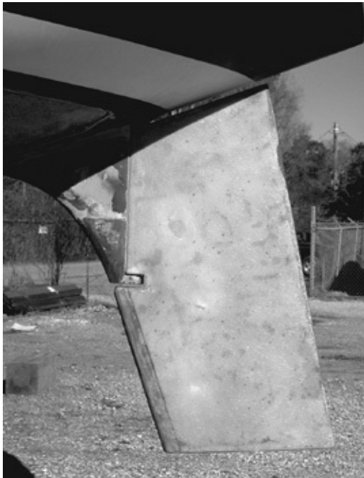
Partial skeg. The lower rudder bearing is an invitation to foul lines.
