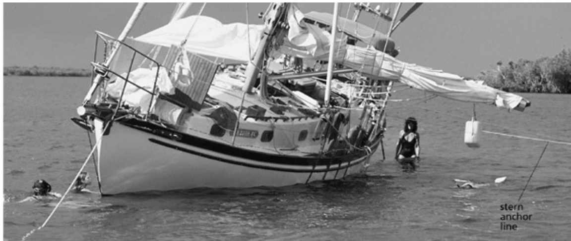
The leverage of the boom can be used to heel a boat.
