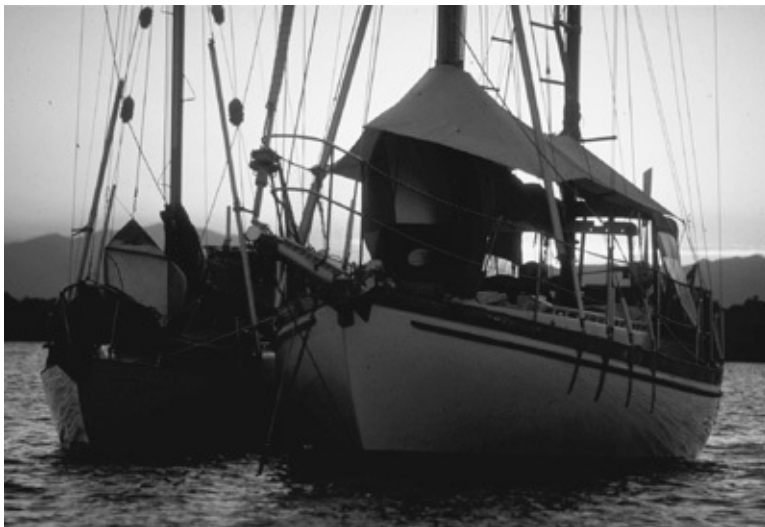
A wind scoop maximizes the airflow through a boat. Notice how this wind scoop bells out to maximize the
