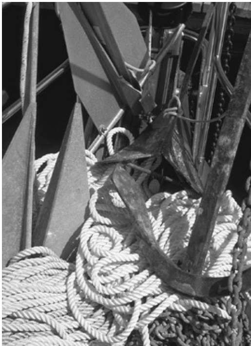
Ground tackle on Nada. This represents a lot of weight, most of it stored well forward.
