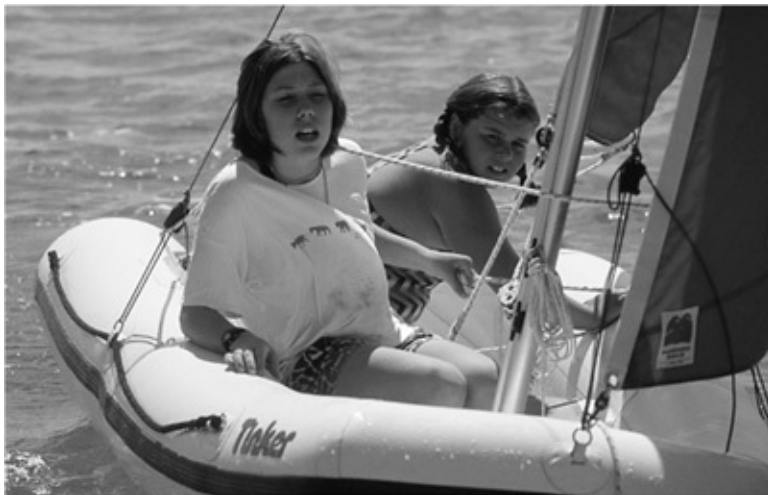
The Tinker folding rigid inflatable in action (as far as I know, the only inflatable that can be sailed; it will even go to windward—just!). It is fun to sail, but as with most of the Tinker inflatables, it has a relatively fine bow that tends to make it a little wet.
