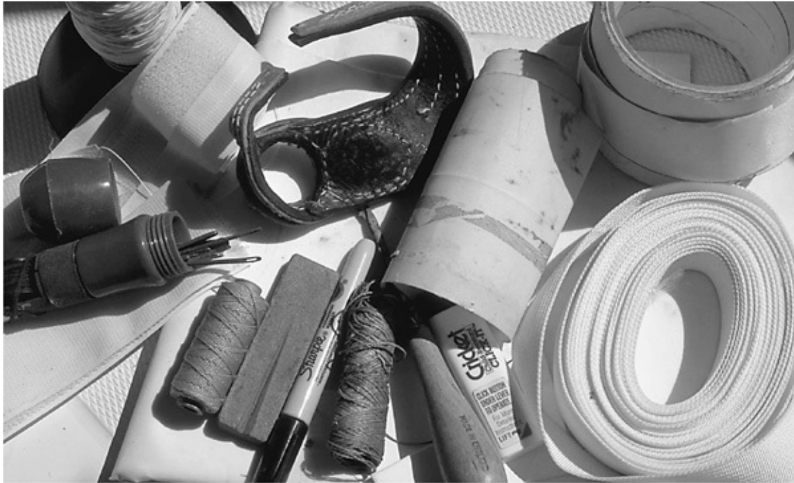
Rudimentary sail repair kit: Dacron thread, Velcro, needles, twine, needle-sharpening stone, sailmaker's palm, cigarette lighter, self-adhesive Dacron tape, nylon webbing, and some scraps of sailcloth.
