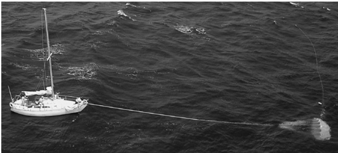
Sea anchor deployed. (Courtesy Para-Tech Engineering)
