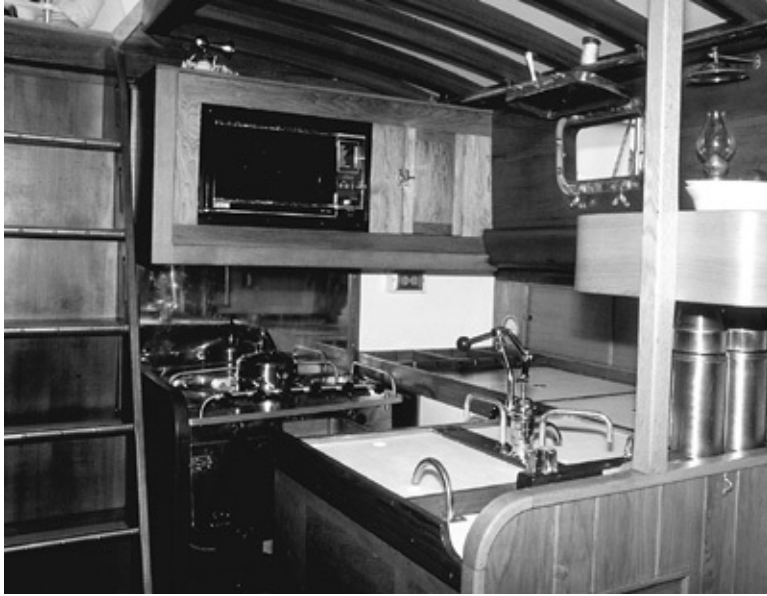
An unusual galley with some truly excellent features. Both the stove (which is gimbaled) and the sinks are mounted athwartships, which is the optimum way to install them. (Courtesy J. E. Paris)
