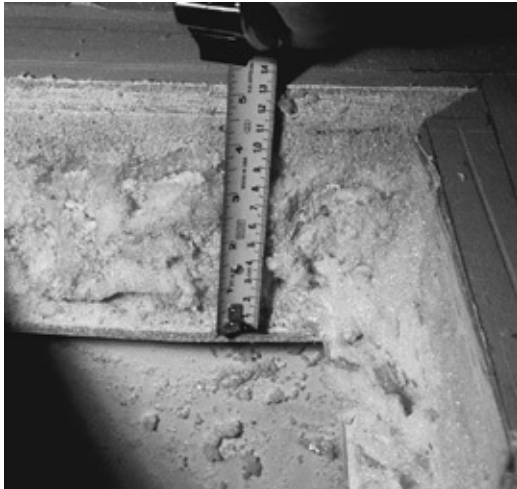
The icebox insulation on Nada is as good as most production boats but, at 4 inches, is not adequate for a freezer on a cruising boat.
