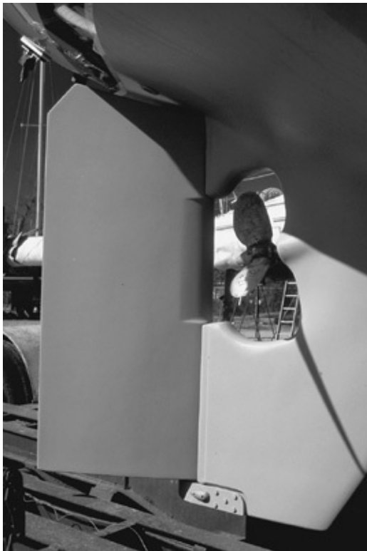
Full skeg on Nada, with the heel bearing at the base of the skeg, and the propeller in an aperture—not the most efficient underbody from a speed perspective, but as close to being bulletproof as possible in a
