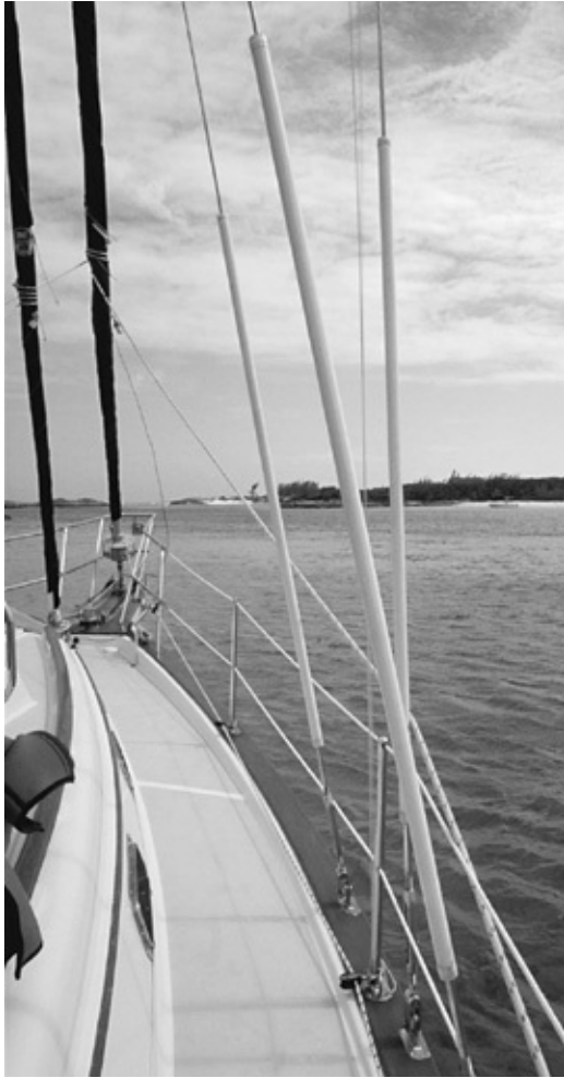
Plastic tubing around the shrouds goes a long way toward minimizing damage from chafe.
