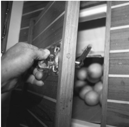
For offshore work, all hatches in the cabinsole need to be positively locked down.
