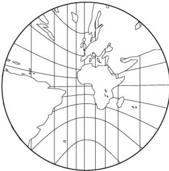
Left: An oblique gnomonic projection. Imagine a light at the center of the globe, projecting outward. Below: Gnomonic projection.
