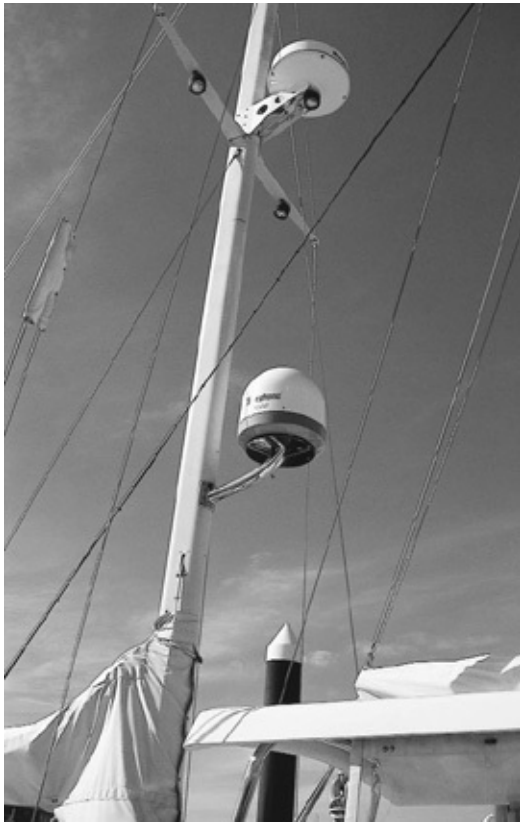
Inmarsat Mini M antenna—note how much smaller this is than an Inmarsat A antenna. (Courtesy KVH)
