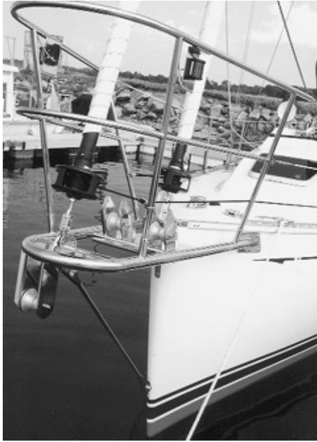
With a plumb stem, a boat needs a bow platform for handling ground tackle. (Courtesy Saga Yachts)
