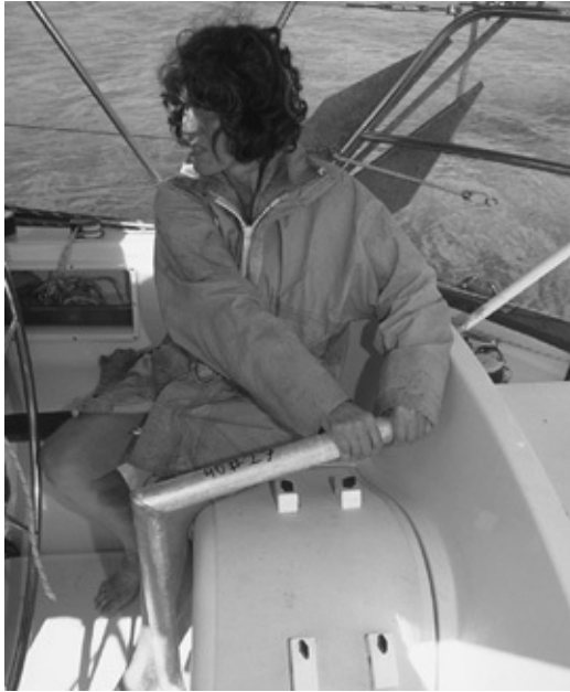
The emergency tiller on Nada—easy enough to fit, but I doubt it has the leverage to steer the boat in much of a seaway.
