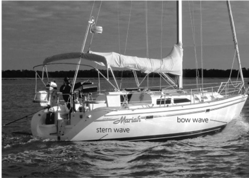
A Catalina 42 doing close to 8 knots under power (speed–length ratio of about 1.34). The crest of the stern wave is just behind the aft end of the boat. Note how cleanly it breaks away from the sugar-scoop transom and how little wake the boat makes.
