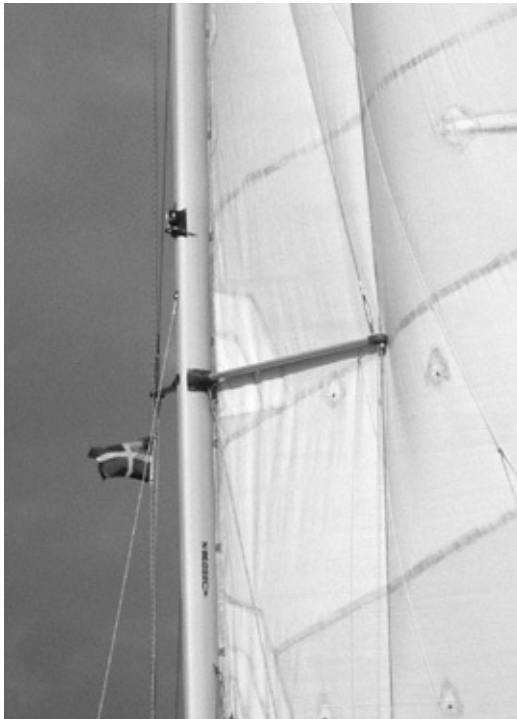
Off the wind, swept-back spreaders significantly limit the extent to which the boom can be let out.
