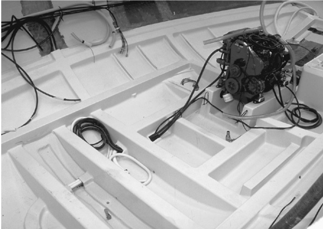
Comprehensive structural grid in a modern boat. (Courtesy Beneteau)
