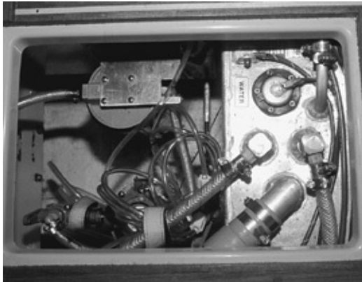
Stainless steel water tank with fittings for the fill and vent hoses, a watermaker, and a tank gauge. The filter is for the watermaker.
