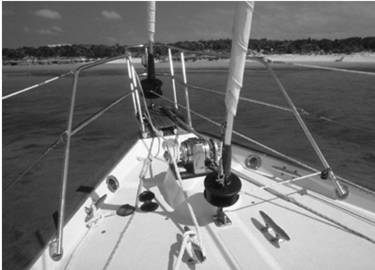
The foredeck on Nada : lots of space to handle ground tackle and plenty of large, well-placed cleats.
