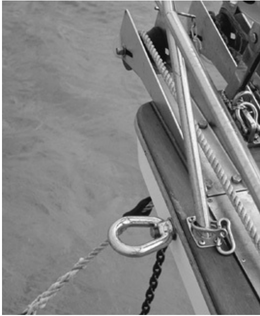
Strong point for the attachment of a snatch block to minimize chafe on a parachute-anchor's rode.
