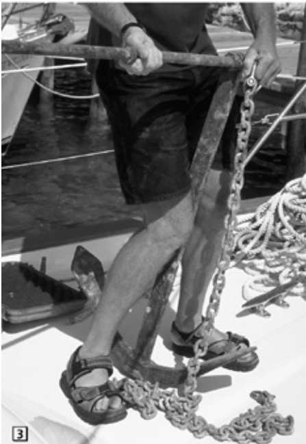
Three-piece 55-pound Luke-style bronze fisherman/yachtsman anchor being assembled. This anchor is our ace in the hole.
