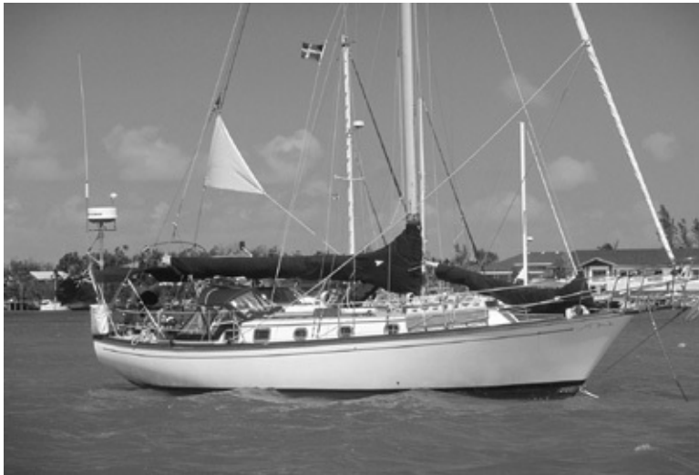
A riding sail. This sail is somewhat on the small side and, as a result, is not very effective. Two or three times the surface area is better.
