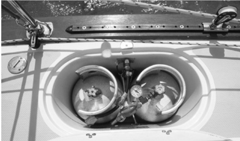
Neat propane installation in a side deck locker. However, water sluicing down the side deck pours into the locker and out of its drain—in time, the salt will corrode the regulator and other fittings.
