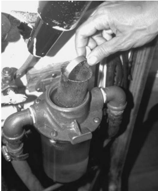
Accessible raw-water strainer. The top is just above the waterline so that it can be opened and cleaned without closing the seacock.
