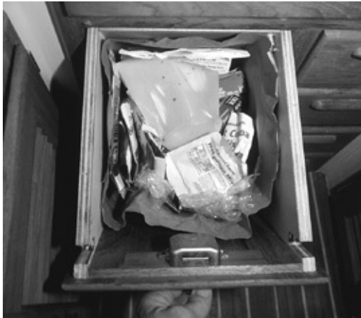
Hinged-out trash bin. It would work better if there were some means of keeping it open (it has to be held with one hand) and some way of attaching trash bags. It is these nit-picky details that ultimately determine the functionality of a galley.
