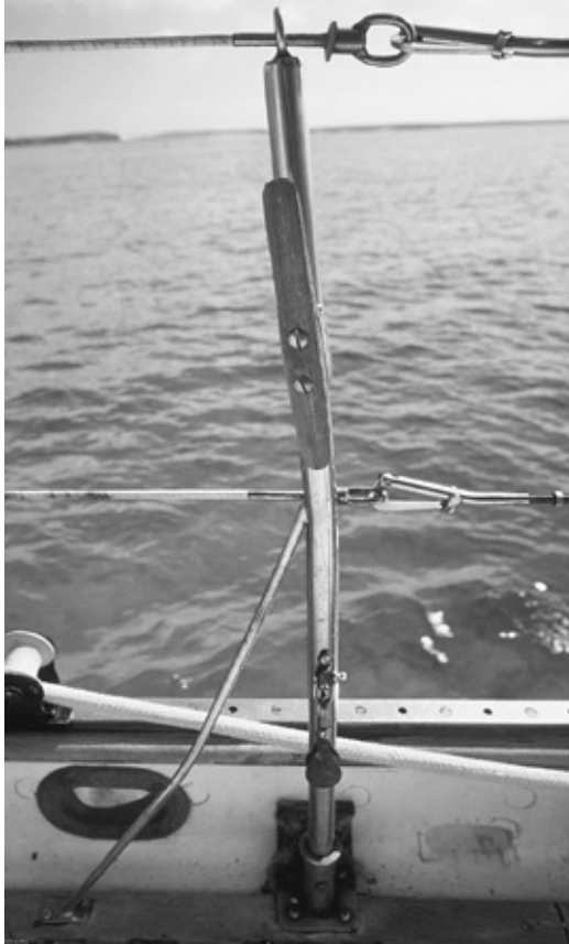
A pitiful gate! The reinforcing strut is completely inadequate to the task, and intersects the stanchion way too low.
