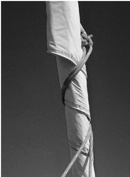
In a high wind, this poorly furled sail will flog, damaging the sailcloth and chafing the stitching.
