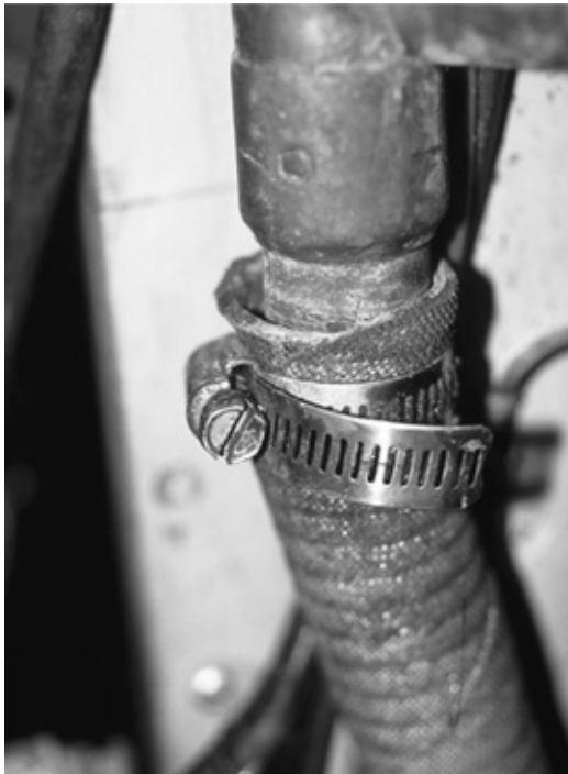
Another fine mess. An oversized hose clamped down with a rusting hose clamp. If the clamp fails, the boat is likely to go to the bottom.
