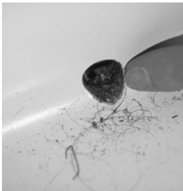
Small limber hole in the structural grid on a modern, flat-bottomed boat (note the staple for size comparison).
