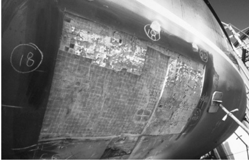
Core damage from running aground. The hull puncture was quite small, but the core damage extensive. The boatyard has been cutting one square after another from the outer skin, looking for the limit of the damage.
