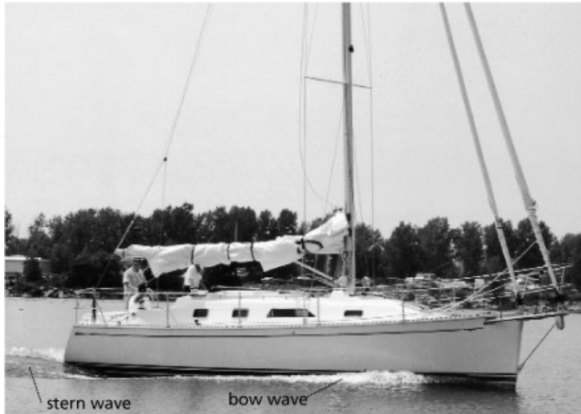
Saga 35 at about 7.5 knots. Again, the crest of the stern wave is just behind the aft end of the boat, breaking cleanly away, and the boat is making remarkably little fuss. (Courtesy Saga Yachts)
