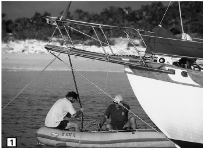
Above: Setting an anchor with a nylon rode from a dinghy—the rode is being dragged out behind the dinghy.
