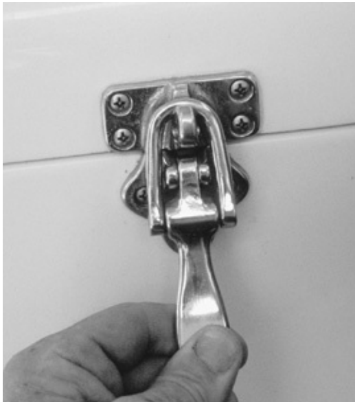
Cockpit lockers need hardware that can stand up to boarding waves.
