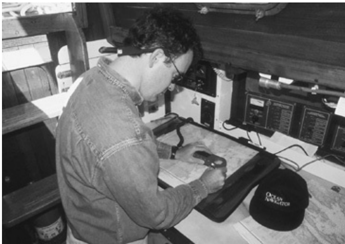
Above left: Yeoman plotter installed in our navigation station. The unit is wired to a hand-held GPS (upper left) with an external antenna. It is relatively simple to move it to the cockpit. Above right: An even more portable (and weather-resistant) version of the Yeoman plotter is this Sport version.
