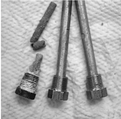
New and old zinc pencil anodes. The old one is at the point where it should be replaced (about half gone).
