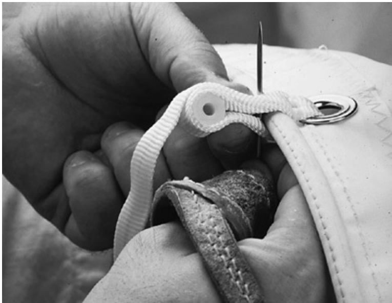
Sail slides should be attached with webbing and sewn rather than attached with shackles. (Courtesy Harken)
