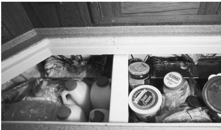
Freezer (on the left) and refrigerator boxes. Neither need be too big—it is better to put any unnecessary volume into more insulation.
