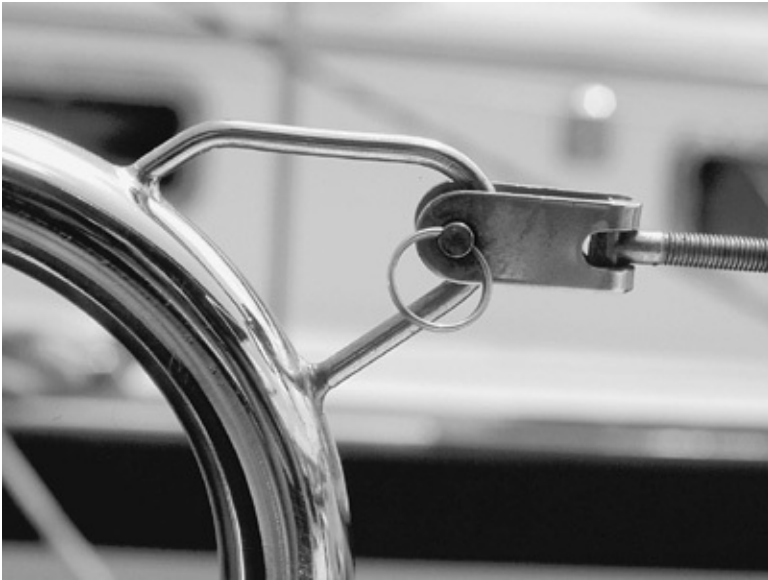
... but with a relatively flimsy attachment for the lifelines. The welds will be easily broken.
