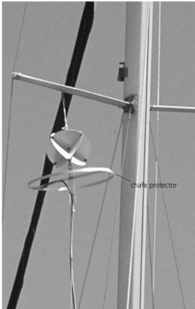
A neat chafe protector on the base of a radar reflector.
