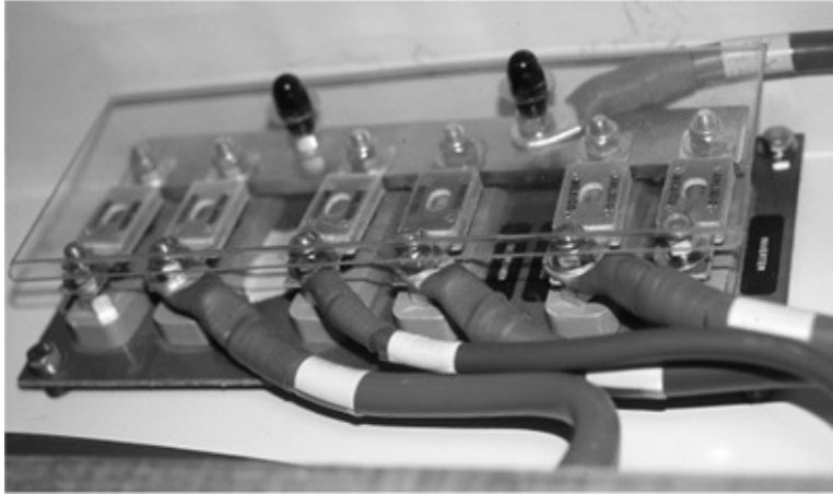
Nada 's high-current bus bar, which is connected to the isolation switch by a short length of cable (see it coming into the bus bar at top right). The high-current circuits are all tapped off this bus bar, via appropriately rated fuses, at left.
