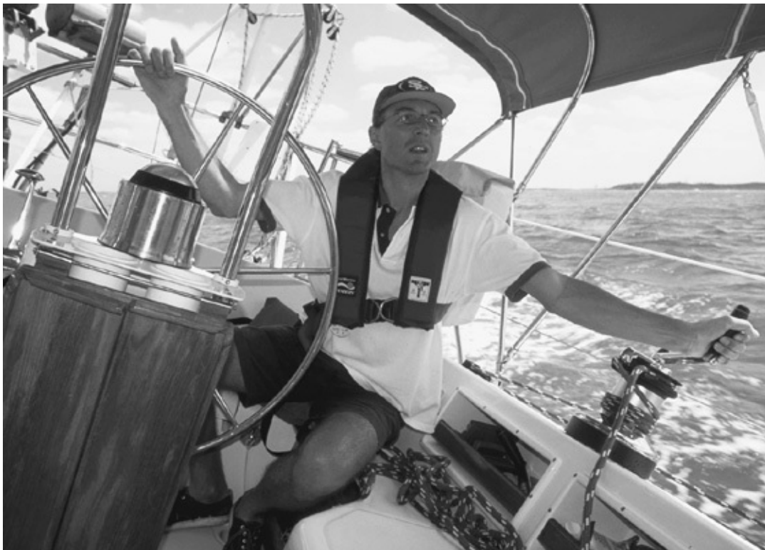
The primary winches should always be accessible from the steering and watch-keeping stations.
