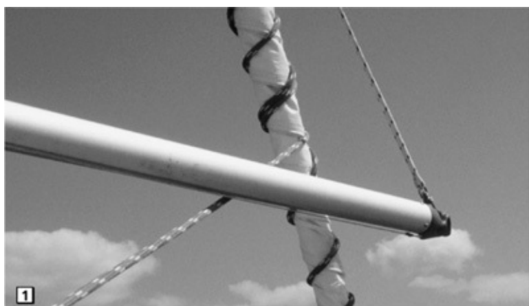
Nada's twin downwind poles, stowed on a track on the forward face of the mast, seen here in the stowed position (hailed up to the top of the track).
