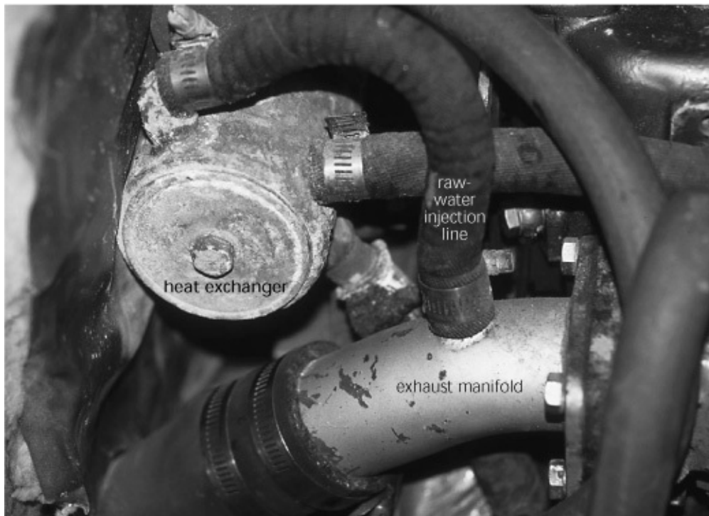
A common sight—the engine raw-water injection line is plumbed directly from the heat exchanger to the exhaust manifold. There is a risk of flooding the engine with salt water.
