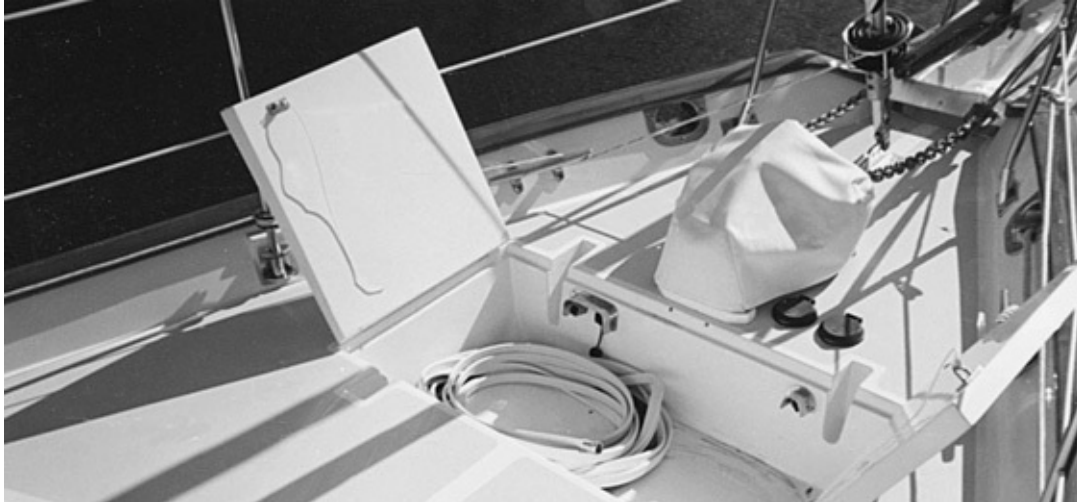
A nice setup, with the chain leading below to a chain locker and an anchor well behind the windlass for stowing a rope rode or other deck gear. (Courtesy Cabo Rico)
