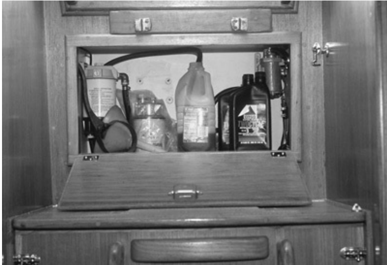
Nada 's filter service station. The fuel-tank vent also comes in here. We place a milk jug under it when refueling, as shown in this photo. This eliminates all possibilities of overboard spills.
