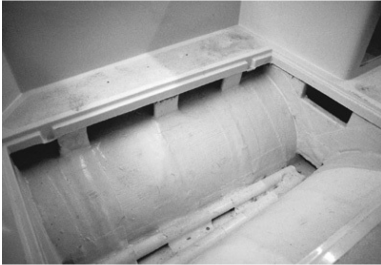
Excellent bonding of interior bulkheads and other components.
