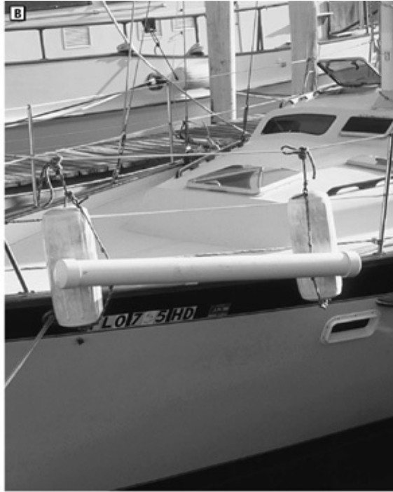
A. Commercially bought rubber end pieces for a fender board; note that one end is breaking up. B. Fender board homemade from PVC pipe. C. This works just as well and is more versatile!
