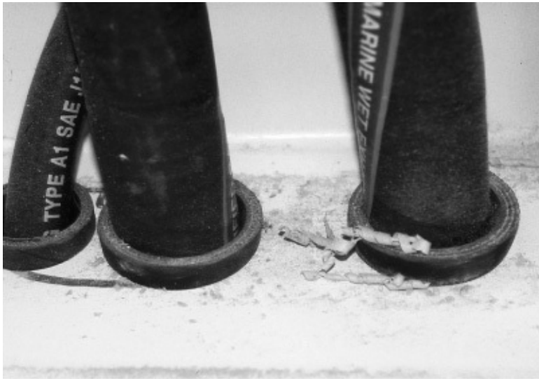
More good hose, beautifully installed to eliminate any possibility of chafe. The fuel-tank vent hose (left) complies with USCG Type A1; the other hose complies with J2006.
