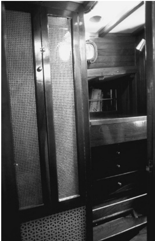
A combination of insulated hull sides, wooden hatch frames, and ventilated lockers such as this one made our old boat just about immune to condensation.
