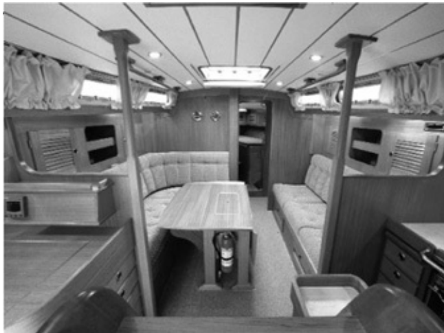
Note the functional navigation station and galley by the companionway, excellent sea berths in the saloon parallel to the centerline, good handholds, and so on. (Courtesy Hallberg Rassy)
