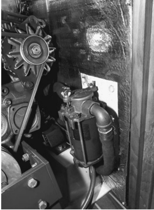
Excellent access to the raw-water strainer.
