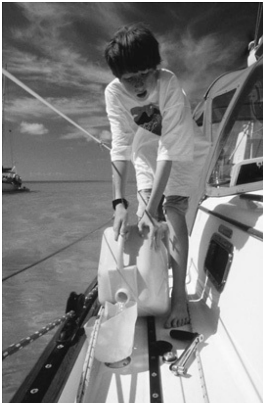
Deck fill fittings need to be located so that a good-size funnel fits in without obstruction. Another couple of inches clearance between the bulwark and the deck would be helpful here.
