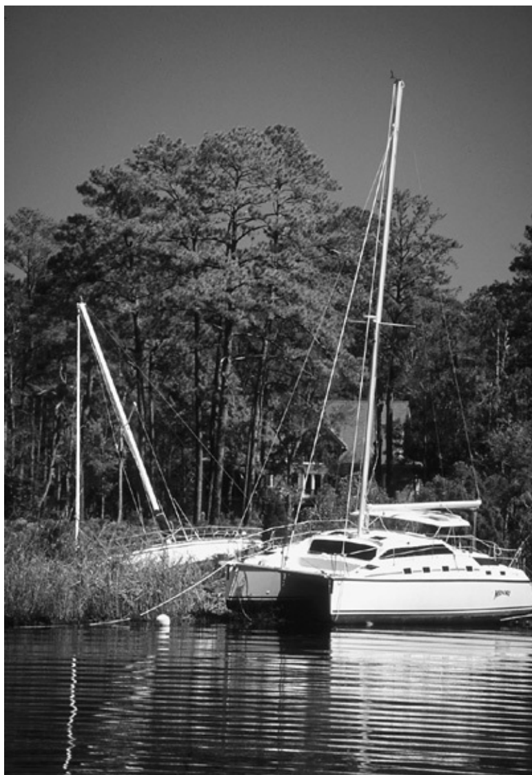
A combination of failed rodes and dragged moorings put these boats on the beach during Hurricane Floyd.
