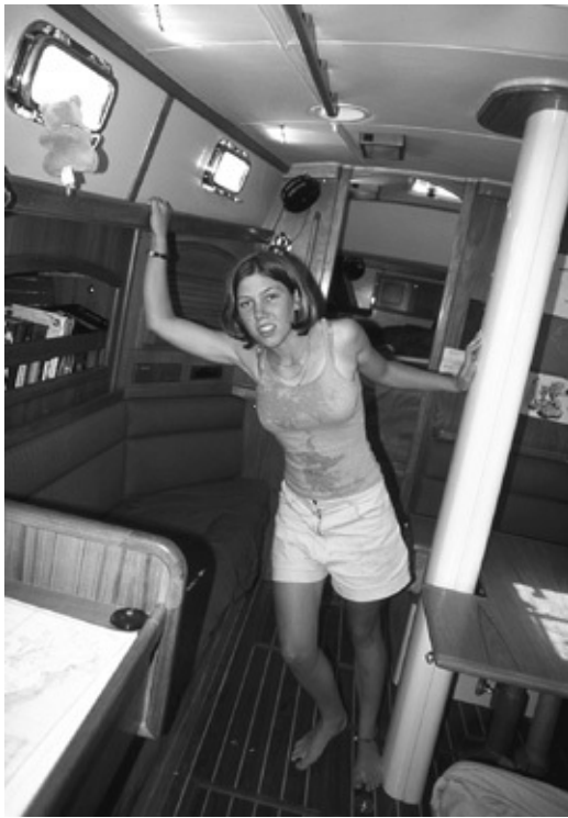
The optimum height for handholds is approximately shoulder height. Overhead handholds are frequently out of reach of shorter crew members.
