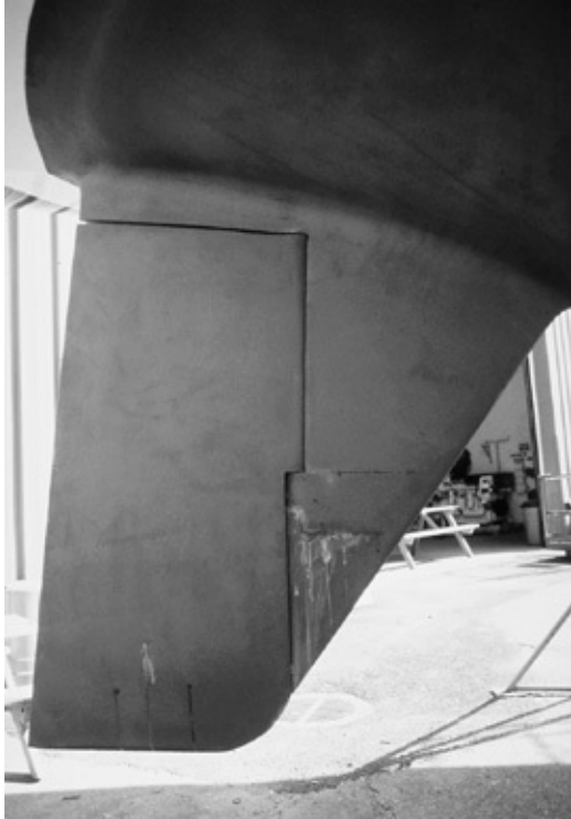
This skeg is angled enough to shed lines, but there is still a risk of something catching between the base of the skeg and the rudder.
