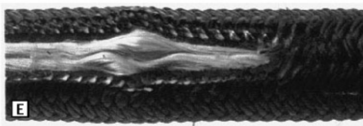
Different kinds of synthetic rope. A. Three-strand nylon. B. Single braid (hollow in the center); rarely found on boats. C. Double braid, which essentially consists of two braided ropes, one inside the other. D. Double-braid construction. E. Parallel core, in which the inner fibers are laid parallel to one another, instead of
