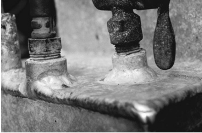
Copper and brass fittings should never be screwed directly into aluminum (as shown here).
