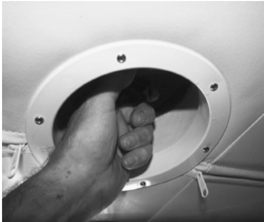
This Dorade vent incorporates a mushroom ventilator, which makes it possible to close the vent from inside the boat.
