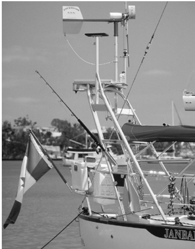
An incredibly elaborate custom-made pushpit that includes mounts for a wind generator, solar panels, a radar, various antennas, an outboard motor and crane, a Lifesling, another rescue throw device, a stern anchor, fishing poles, and probably several other things I have missed!
