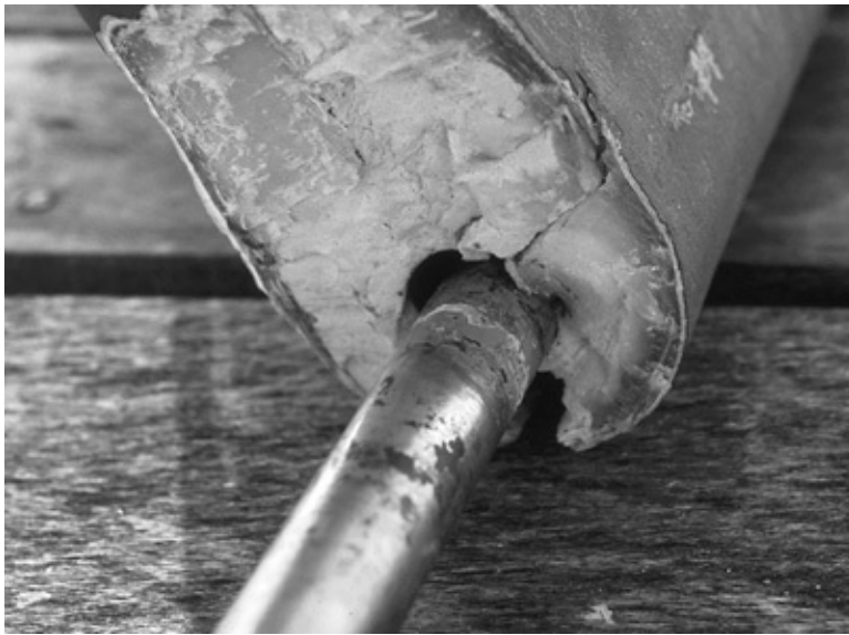
This boat hit a reef and was washed over the top. The boat did fine, but the spade rudder was seriously damaged. A skeg-mounted rudder would likely have survived.
