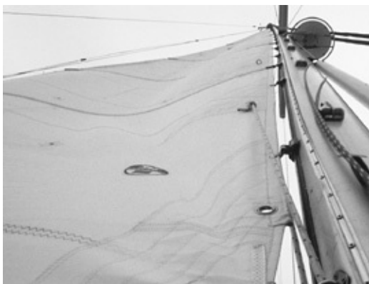
Even head-to-wind, a fully battened sail ripples as opposed to the flogging that occurs with a regular mainsail.
