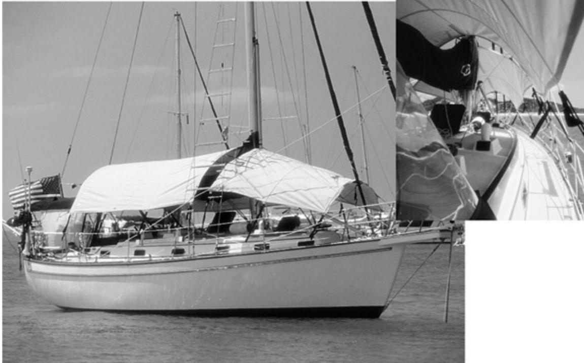
An excellent awning (manufactured by Shadetree of Elberta, Alabama) that has sufficient curvature to enable people to move around on deck, but yet comes down low enough at the sides to create effective shading.
