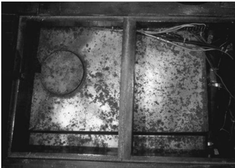
Given unfavorable conditions, most grades of stainless steel used in boat tanks will also corrode, some worse than others.
