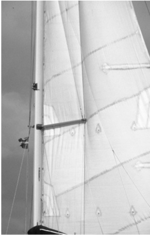
Swept-back spreaders are a liability on a run.
