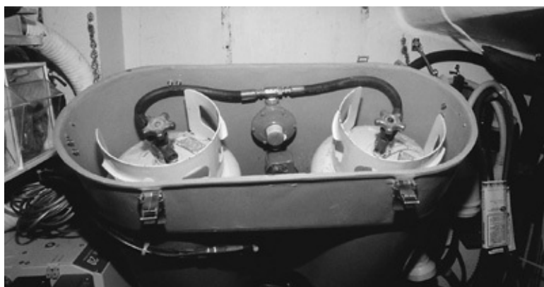
Two different approaches to retrofitting an LPG stove. One is to add a deck box for the cylinders (below ), the other to add an off-the-shelf, sealed LPG locker to a cockpit locker (bottom ).
