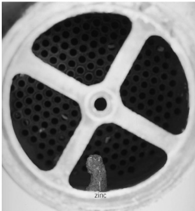
The zinc in this heat exchanger is almost all gone and is virtually worthless. The heat exchanger is at risk of galvanic corrosion.
