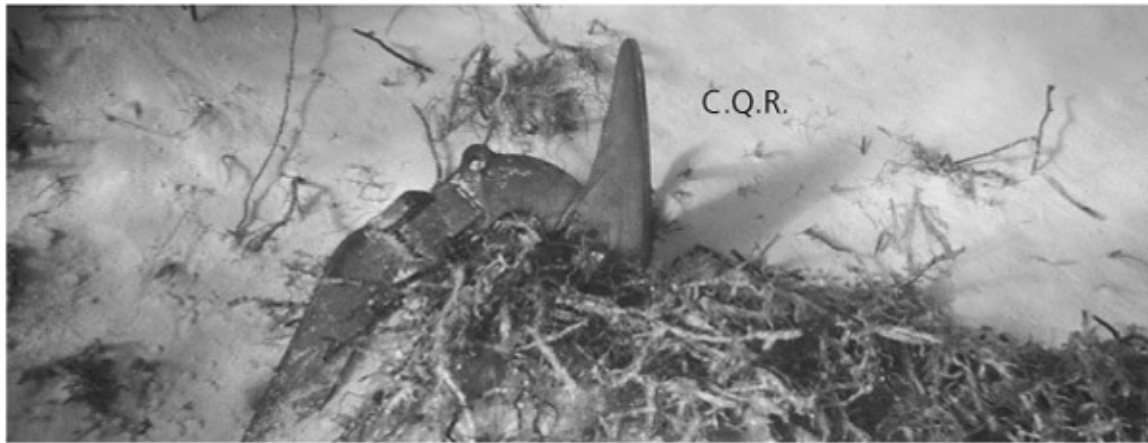
Delta and C.Q.R. anchors about to set. Note the weed fouling the C.Q.R.—it will have little effect on the anchor, whereas if it got wrapped up in the flukes of a Danforth-type anchor, it might impair the set.
