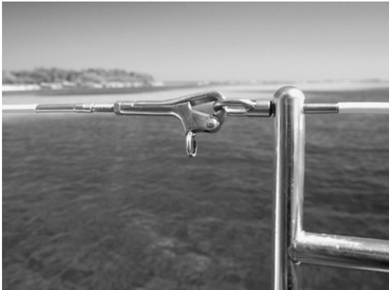
Pin-type pelican hook—this is unlikely to open accidentally.
