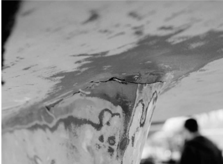
Look for cracks around the root of the keel, especially on boats with fin keels.
