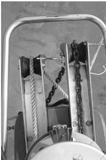
Solid double bow rollers that, nevertheless, still do not allow a Danforth-style anchor to be stowed with a plow-type anchor.
