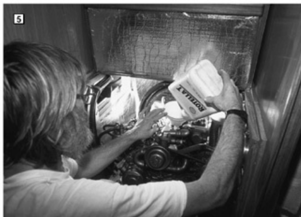
1, 2. Checking and changing the oil on Nada. 3. Note the oil-change pump and the use of a plastic storage bag... 4. to contain the mess when removing the filter (diapers also work well). I would like to have the filter remotely mounted and hanging down (rather than mounted horizontally on the engine)—it would be even easier to change, with no mess. 5. Adding oil.
