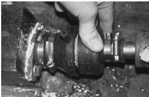
After launching, mechanical seals should be pulled back to allow the seal to flood.
