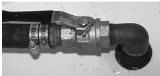
A stainless steel ball valve mounted to a bronze through-hull and elbow with a bronze tailpiece, something I
