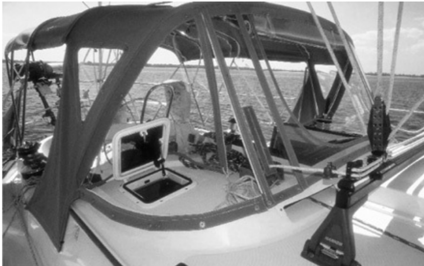
To get good ventilation in our quarter berth, we sacrificed a cabintop winch, installed a hatch, and designed the dodger to wrap around the hatch to form a small wind scoop.
