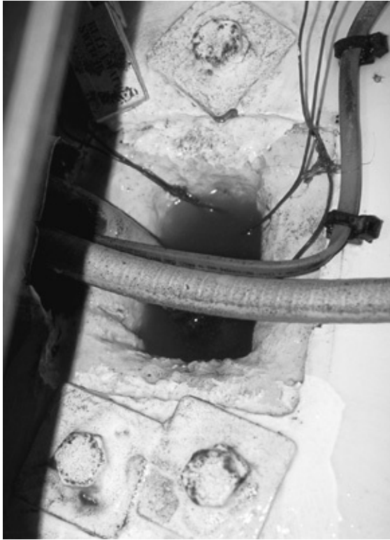
Minimal bilge on a modern, flat-bodied, lightweight production boat. This is still better than some boats that don't have any kind of a bilge sump!
