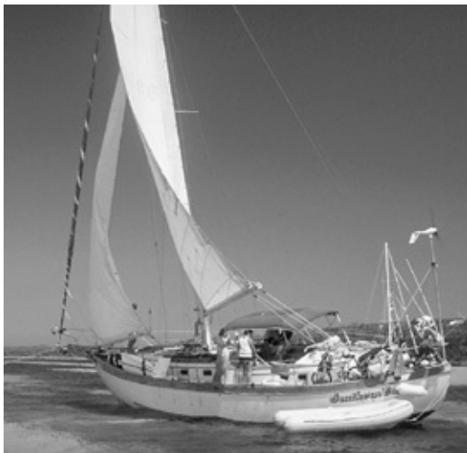
The sails are set to heel the grounded boat. They need to be sheeted in for the most effect.
