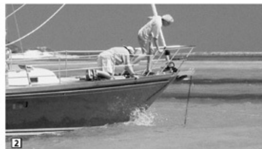
If the anchor rode is let out in a hurry, it may pile up on the anchor and foul it (especially a Danforth-type anchor).
