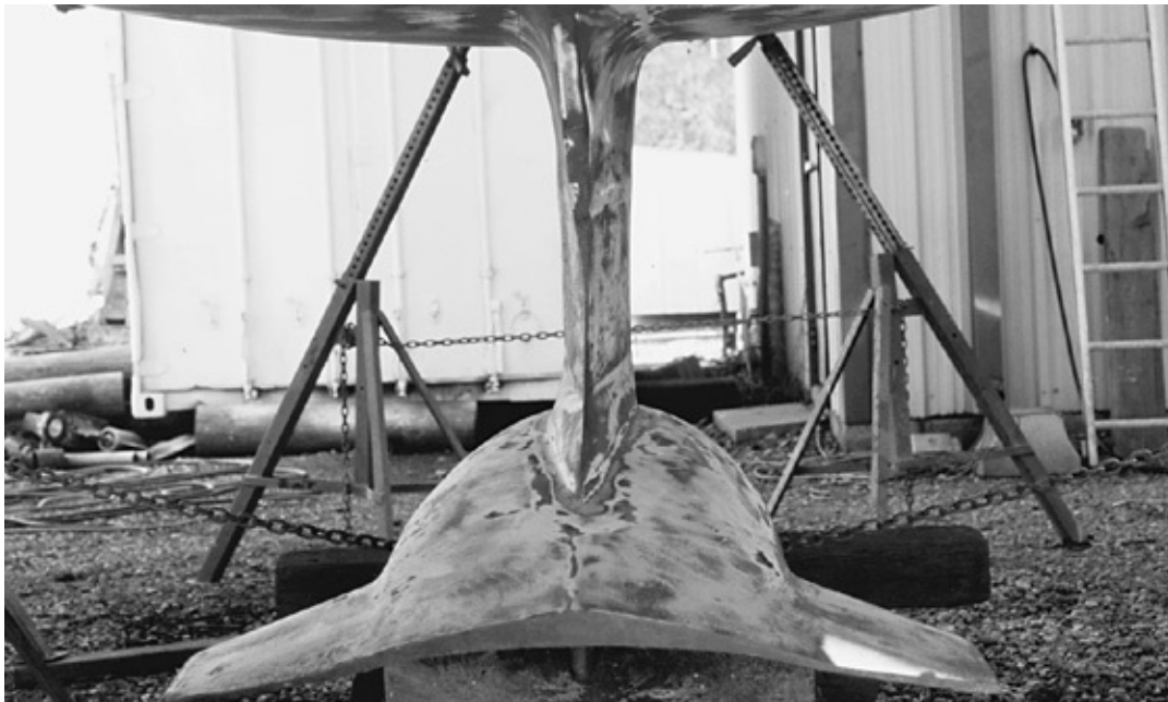
A modern wing keel. Although wing keels have performance benefits, they can be a distinct liability in a grounding.
