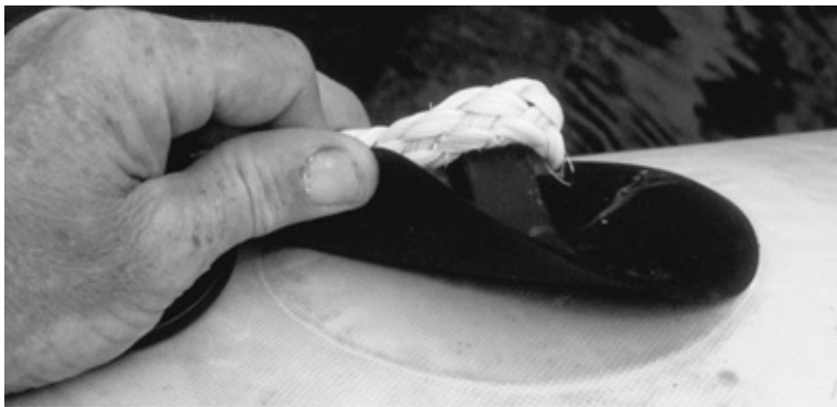
Below: Leaching plasticizers have made this PVC dinghy sticky (hence the shoe marks). Bottom: As the plasticizer leaches out of PVC, it loosens the glue bond with various fittings that start to come loose.
