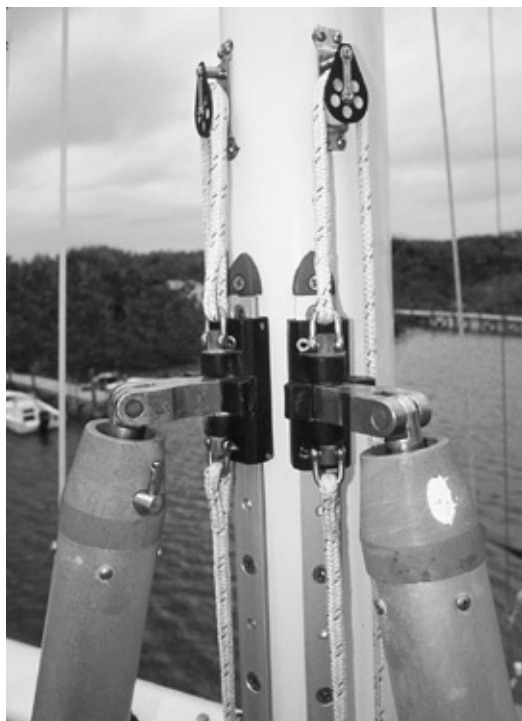
Nada's twin downwind poles, stowed on a track on the forward face of the mast, seen here in the stowed position (hailed up to the top of the track).
