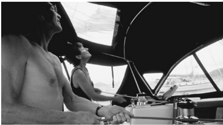
Single-line reefing. The person in the foreground is easing the halyard while the crew member in the background cranks in the reef. No one needs to leave the cockpit.
