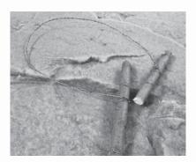
Improvised wire saw with two pieces of twisted wire
