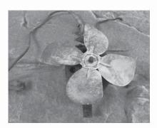
File this old fan blade to make a suitable cutting tool
