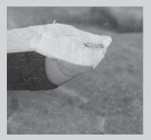
Close-up of chisel tip (A)
