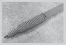
Step 4: Pull the tag end sticking out of the bottom. This will pull the loop around the tail and under the wrapping. Trim the ends.
