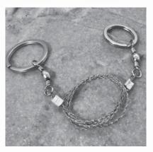
Commando wire saw (the better of the wire saw models)
