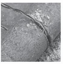
Close-up view of the twisted wire cutting through wood
