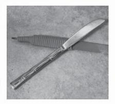
Butter knife filed to make a sharp cutting tool using a simple file
