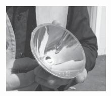
Flashlight reflector burning an ember into a piece of punky wood (the tinder is held through the hole in the bottom, and the focal point is very close to the bottom)
