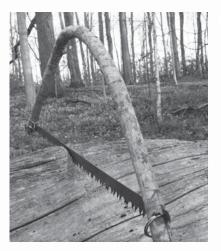
Close-up of a key ring used to help hold blade in place
