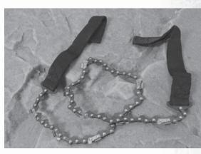
Wire-style saw with chain saw blade
