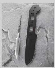
A comparison of a partial tang blade (left) and a full tang blade (right)
