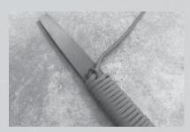
Step 3: When you reach the loop or run out of cordage, run the tail through the loop.
